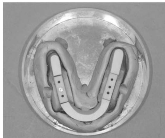
Fig. 2. Mandibular phantom made using the bone blocks and radiopaque acrylic resin
